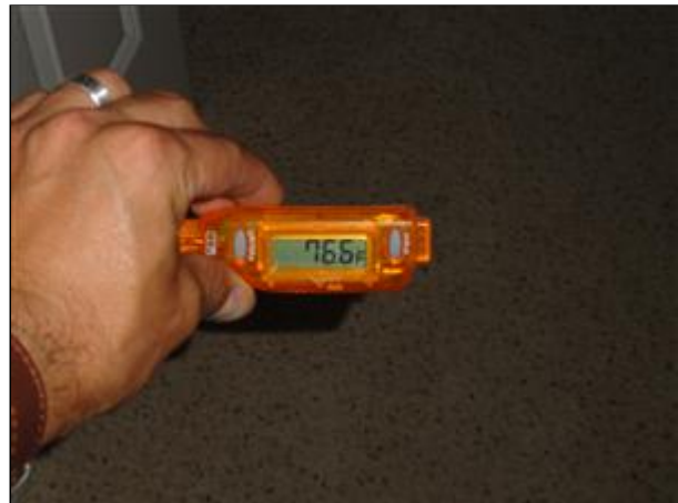
Item 23 - Picture 2 elevated 2nd fl temp (insulation/ventilation also a role)
