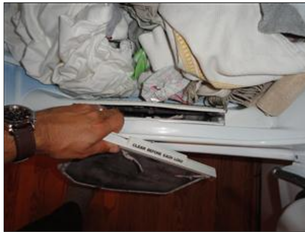
Item 50 - Picture 1 clean lint passages
