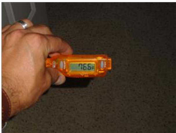
F. Picture 2 elevated 2nd fl temp (insulation/ ventilation also a role)
